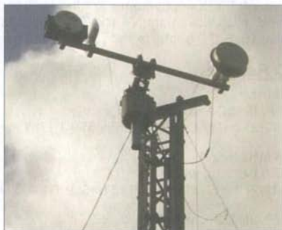
76 GHz Radar station antenna at LX1DU
