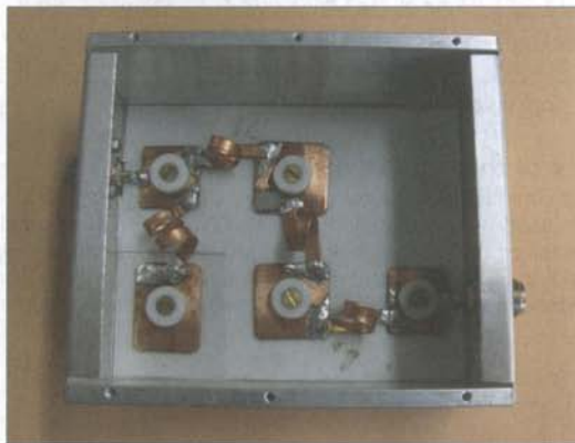
Fig. 5: 70cm KW Low Pass Filter by F5CYS
